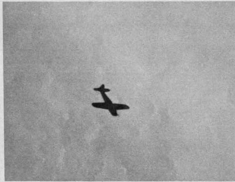
JUDY Low but lengthy greenhouse provides good visibility for Judy's two-man crew on reconnaissance flights from Japanese carriers. The fuselage is long in proportion to wing,
